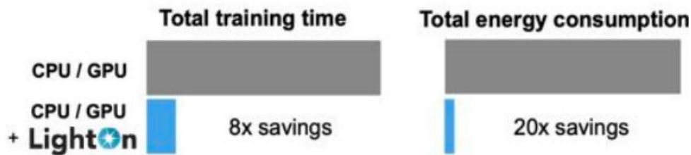
Figure 5: Typical benchmarks for the OPU, in time and energy, on a whole Transfer Learning training task. Starting from a pre-trained VGG16 Deep Neural Network, the task is to specify the classification layers to the STL10 database.
